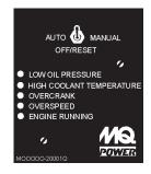
Figure 44. Engine Running LED (ON)
